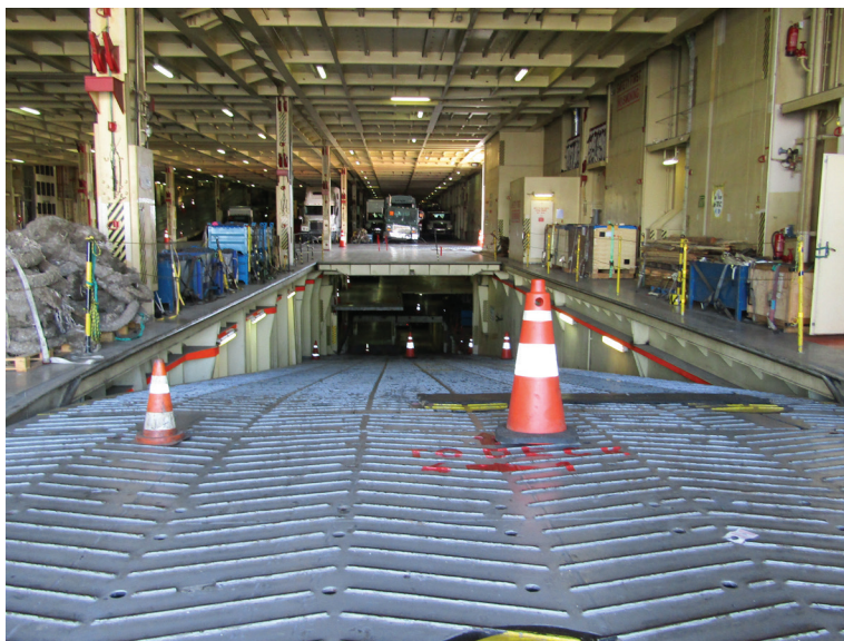
Auto ramp between decks on the car carrier
