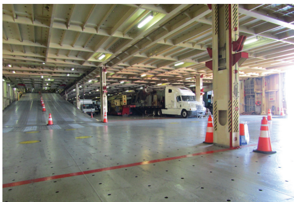
Ramps lift to seal each deck level
