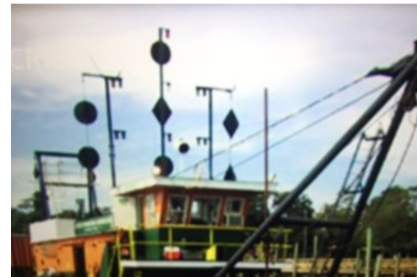
Vessel showing RAM day shapes in center. The two balls indicate the obstruction side and a vessel should pass on the side showing the two diamonds.
