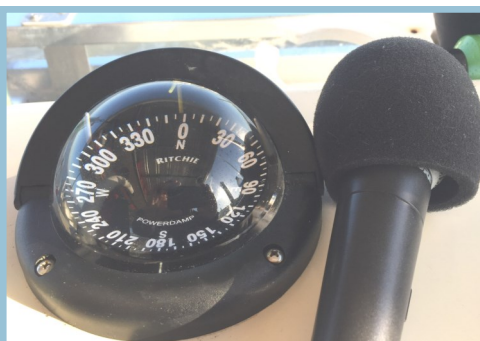
Compass reading 355°. Public address microphone is pulling 20°WEST.
