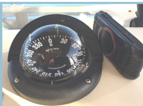
Compass reading 015°. Flip phone is pulling 40°WEST.
